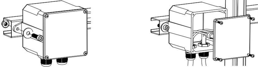
**Step 4. Attach the APsystems microinverters to the racking or the PV module frame.**
