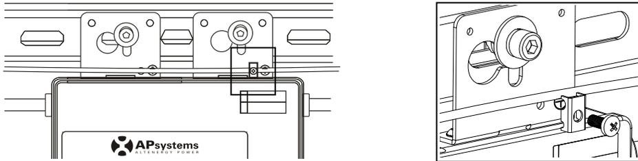
**Step 8. Place the PV modules and connecting each YC500 to the two PV modules close-by.**
