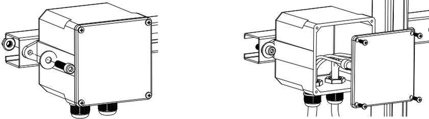
**Step 4. Attach the APsystems microinverters to the racking or the PV module frame**
