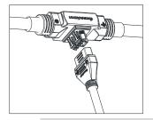
NOTE: Cover all unused T connectors with sealing caps to protect the T connectors.
