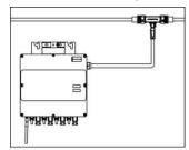
NOTE: AC connector interface as follows, from left to right PE, N, L3, L2, L1.
