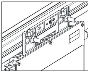
**Step 4. Attach the antenna to the microinverter, and keep the antenna vertical to the earth.**
