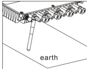
**Step 5. Connect the APsystems Microinverter cables to the AC bus cable.**
