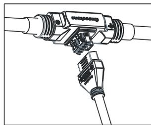
*NOTE: AC connector interface as follows, from left to right PE, N, L3, L2, L1.*
