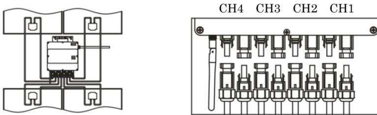
**Step 7. Install a protective end cap at the end of AC bus cable.**
